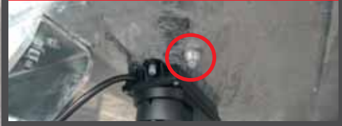
ANTI-THEFT BOLTS SECURING THE PRESSURE WASHER TO THE CHASSIS
