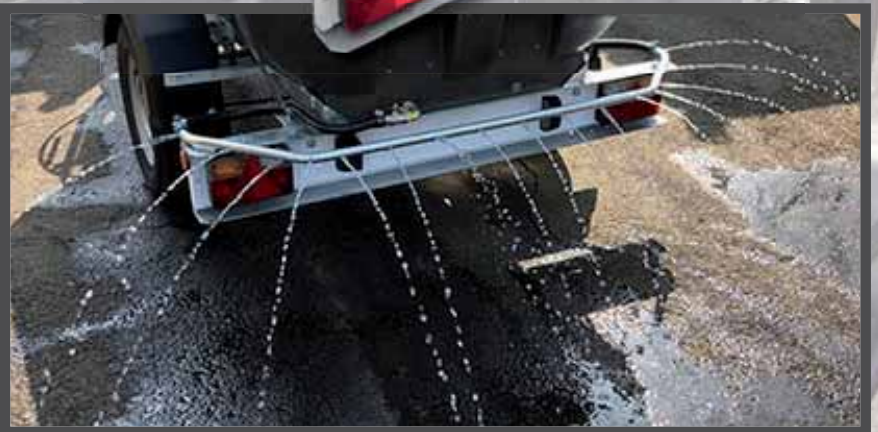
GRAVITY-FED SPRAY BAR OPTION FOR DUST SUPPRESSION
