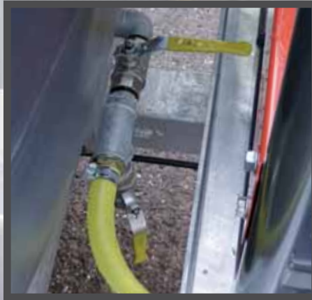
TANK AND PUMP DRAIN TAPS FOR SAFE TRANSPORTATION & PREVENT FROST DAMAGE
